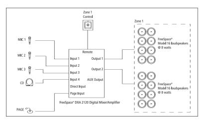
(1) Mixer Mode – Each input can be routed to every output simultaneously. The simple front-panel control allows easy gain adjustments for up to four microphones. Control volume for each channel independently, or use master volume to control both outputs at the same time.
