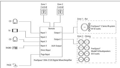
(2) Dual Mono Select Mode – Two input sources are available for each output channel. Volume control and source selection are available in each zone.
