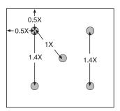
For linear spacing (for bordering sidewalks, paths or walkways): Use the ratios shown above left, keeping the speaker at least 3 ft (1 m) from the listeners.
